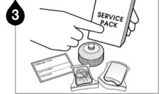
Check the grease pouch capacity and the service pack items (battery pack, grease pouch & dust cover).
