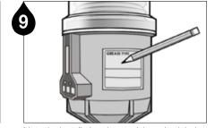
Note the installation date and the scheduled completion date of lube cycle on the lubricator using the label provided in the Service Pack for maintenance purposes.
